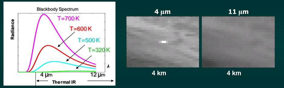
**Planck's Law:** Radiance  $(\lambda) = B(\lambda, T)$ wavelength temperature fire R<sub>4µm</sub> >> R<sub>11µm</sub>
